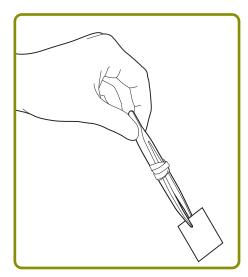
Oip the circuit board into the iron(III) chloride solution to etch the board. Make sure that the entire board is covered. Gently swirl the solution occasionally.
