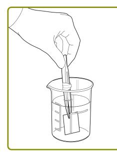
After 10 minutes start checking the board to see if etching is complete. Remove the circuit board and dip it into clean water in a plastic tray. Look to see if the copper that is not protected by the photoresist is completely etched away, revealing the plastic underneath. If the copper is not completely etched, place the board back into the solution.
